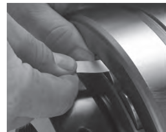
Fig. 95. Measure of RIC before installation.
