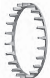
Fig. 46. Split, machined-brass, land-riding, finger-type cage.
