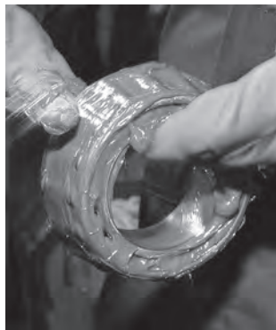
Fig. 147. Grease can easily be packed by hand.
