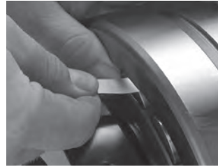
Fig. 91. Measure RIC before installation.
