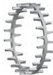
Fig. 44. One-piece, machined-brass, roller-riding, finger-type cage.
