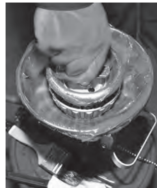
Fig. 148. Mechanical grease packer.
