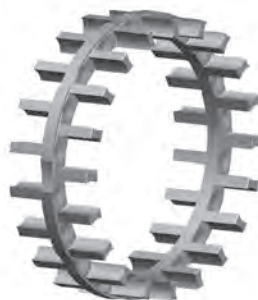
Fig. 49. One-piece finger-type cage.
