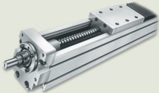
Runs with high positional accuracy: Linear actuator with monorail guidance system and integrated spindle drive – spindle is covered by bellows – medium to high loads can be moved with high precision
