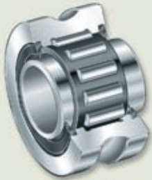
Profiled track roller (non-locating bearing): Needle roller bearing with profiled outer ring and movable inner ring – can be used combined with guideways
